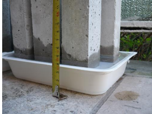
Figure 6. – Concrete specimens without hydrophobic coating
