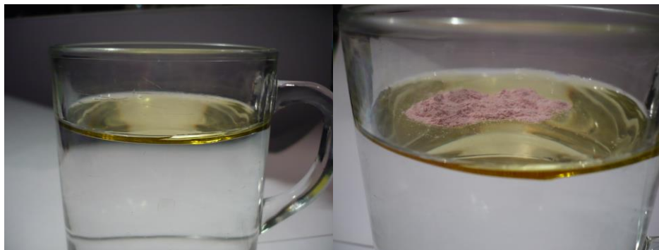
Figure 8. – Oil pollution on left picture (olive-oil), right picture oil with hydrophobic material
