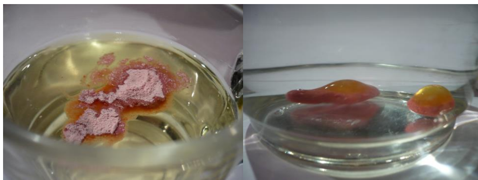
Figure 9. - The olive oil will be adsorbed and the oil- SG-air is sinking on the bottom
