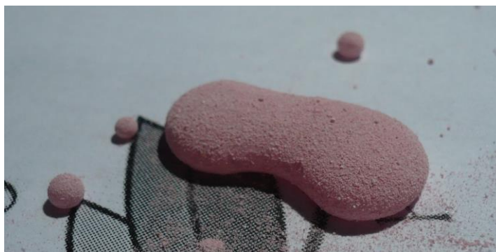
Figure 5. - Drops of a water suspension of the hydrophobic admixture on a surface of a paper
